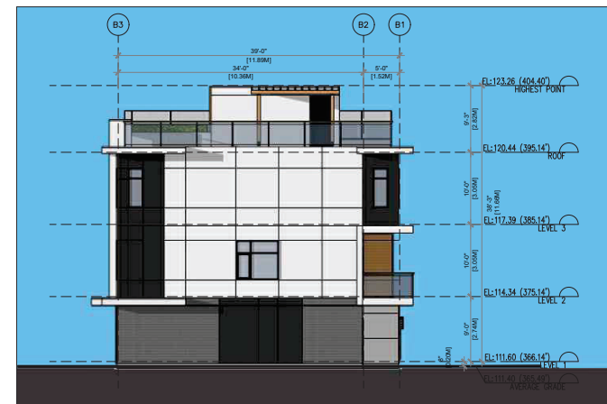
BLDG B NORTH ELEVATION
