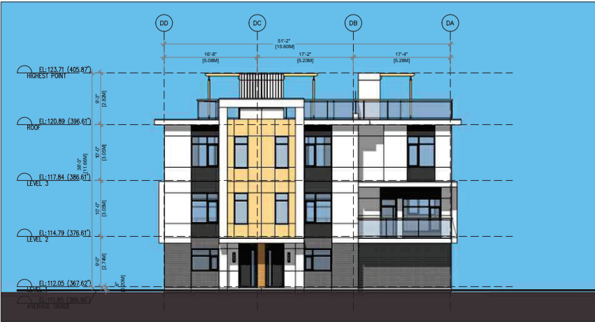
BLDG D EAST ELEVATION
