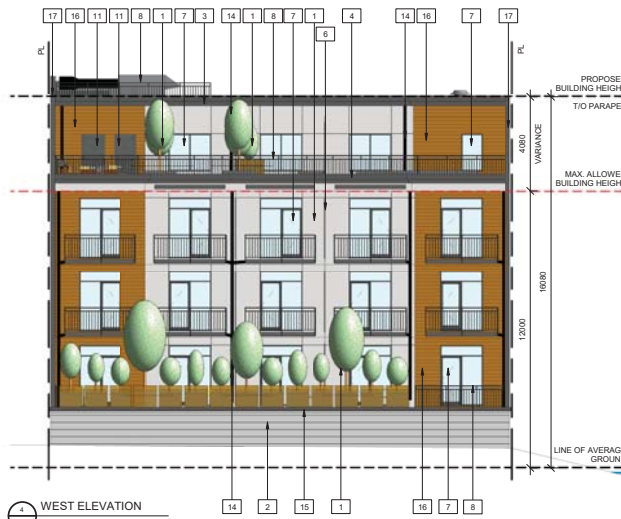
4 WEST ELEVATION DP3-1 1:100
