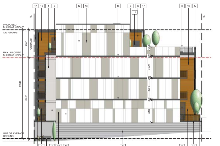
3 NORTH ELEVATION DPS-1 1:100
