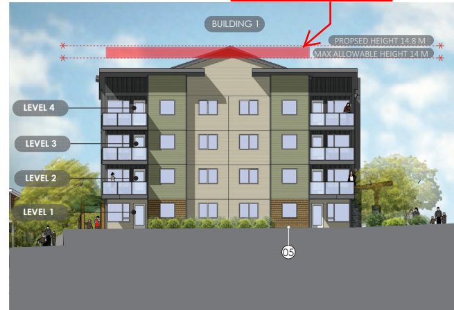
BLDG 1 | EAST ELEVATION | Scale 3/32" = 1' |
