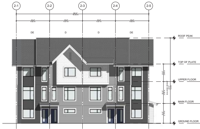
1 SOUTH ELEVATION - BUILDING 2 & 17 1:100
