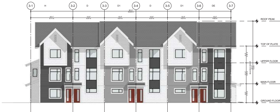
1 SOUTH ELEVATION - BUILDING 3 & 16 1:100
