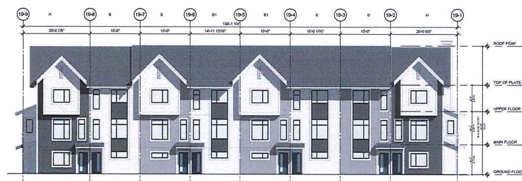
4 BUILDING 19 WEST ELEVATION 1: 100
