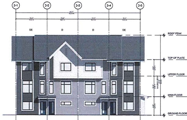
1 SOUTH ELEVATION - BUILDING 2 & 17 1:100
