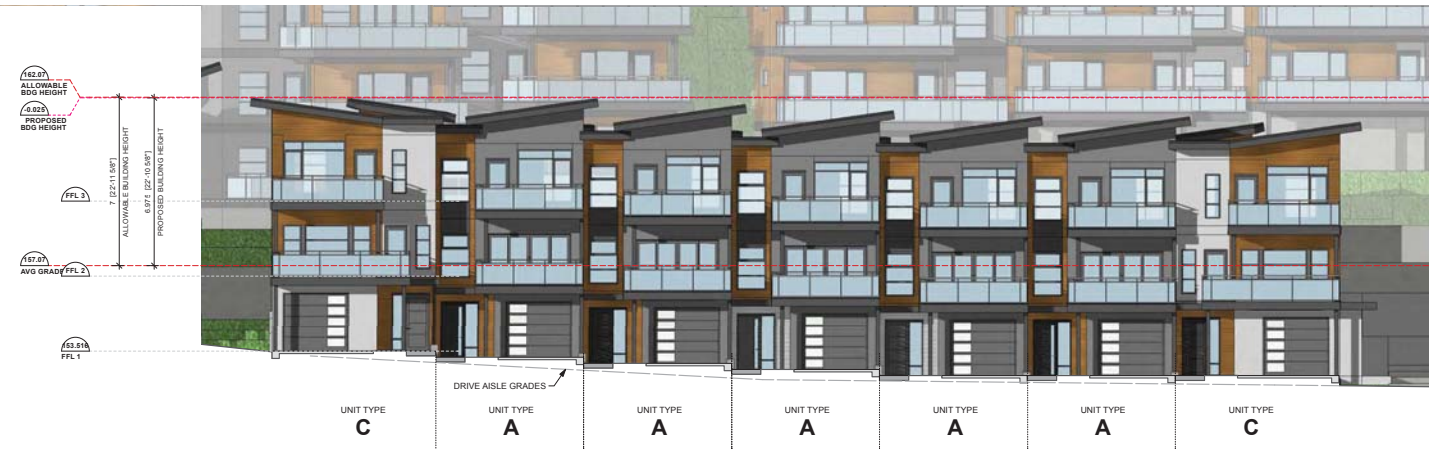
3 Building 7 Street Elevation Scale: 1/8" = 1'-0"
