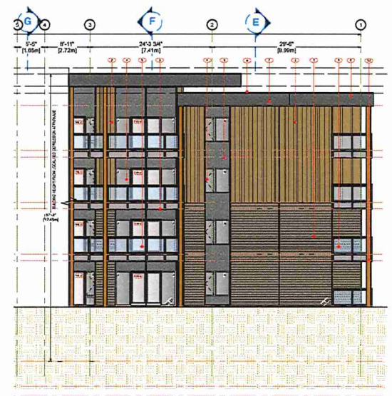
3 North Courtyard Elevation 1/8" = 1'-0"
