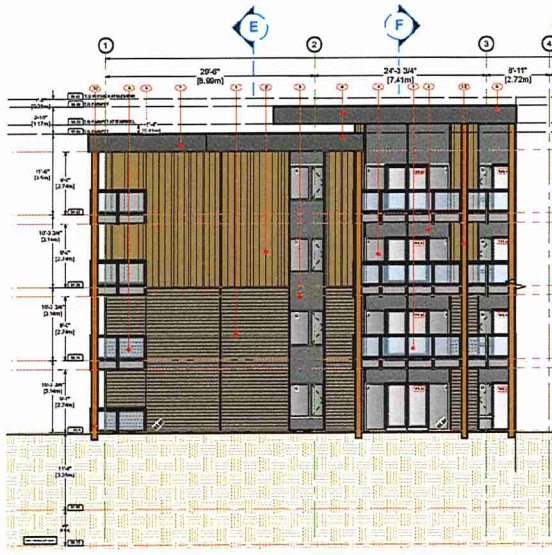
1 South Courtyard Elevation 1/8" = 1'-0"
