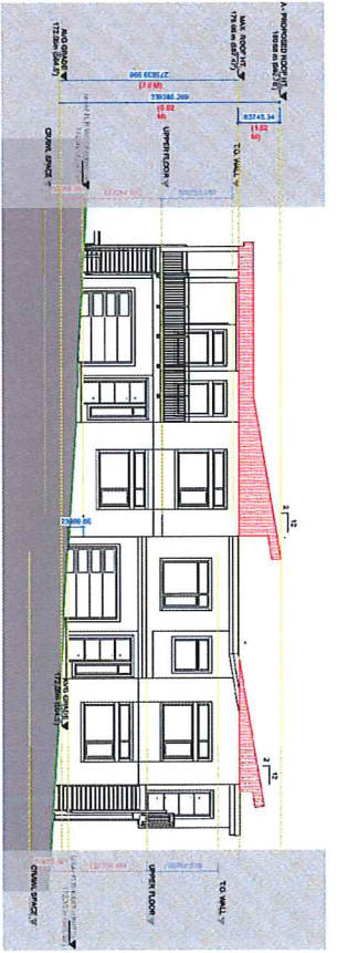
BUILDING A: SOUTH ELEVATION PROPOSED HT.: 5.82 M. MAX. HEIGHT: 7.00 M HEIGHT VARIANCE REQUESTED: 1.182 M
