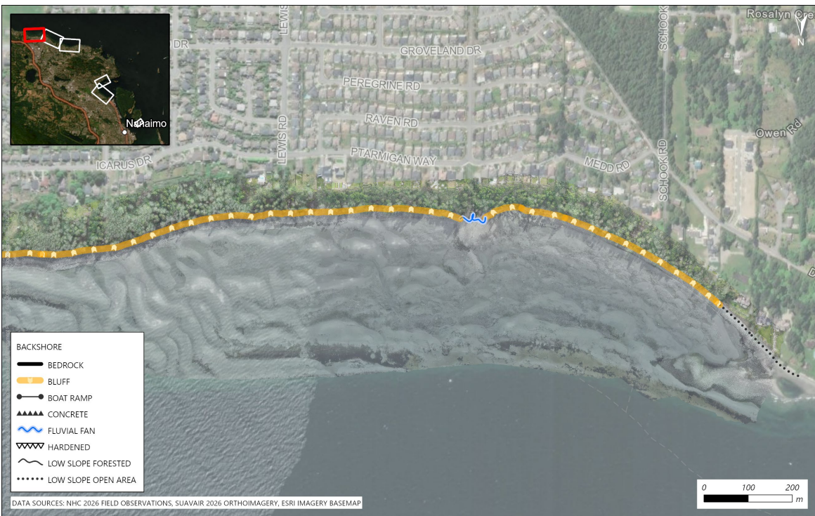
Figure 3.5 Backshore morphology mapped along the west side of the North Shore focus area.
