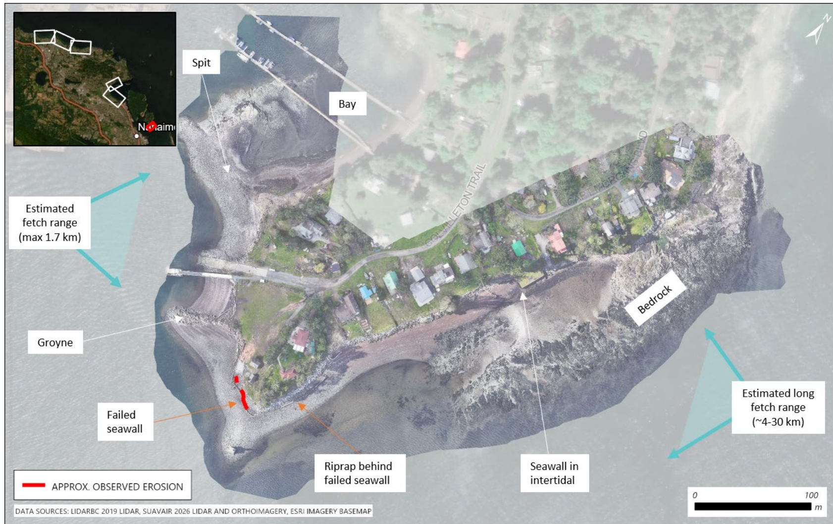
Figure 3.16 Map of observed features and areas of active erosion within focus area on Protection Island.
