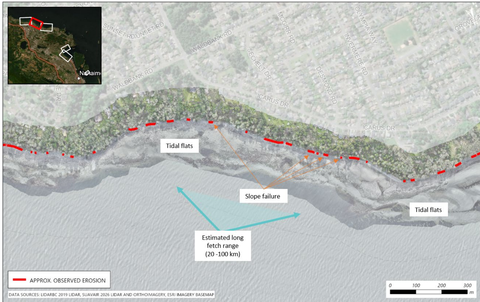
Figure 3.2 Map of observed features and areas of active erosion along the center of the North Shore focus area. Slope failure locations are approximate.
