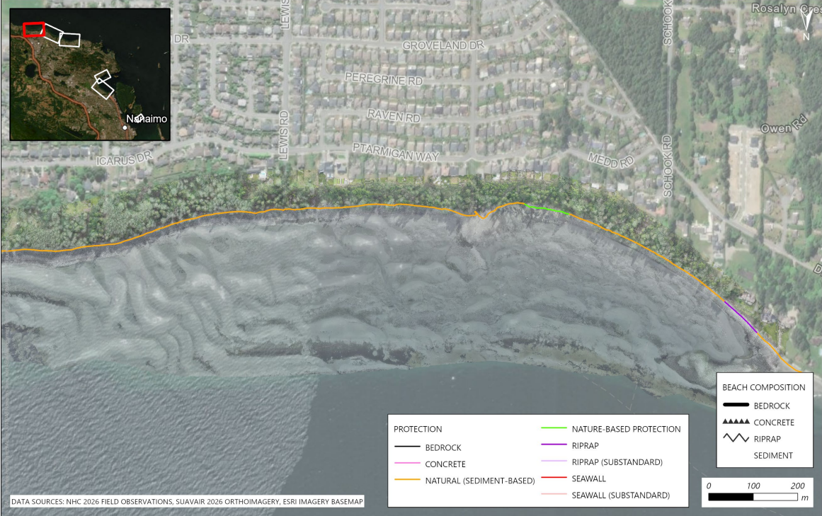
Figure 3.4 Shoreline protection and beach composition mapped along the west side of the North Shore focus area.
