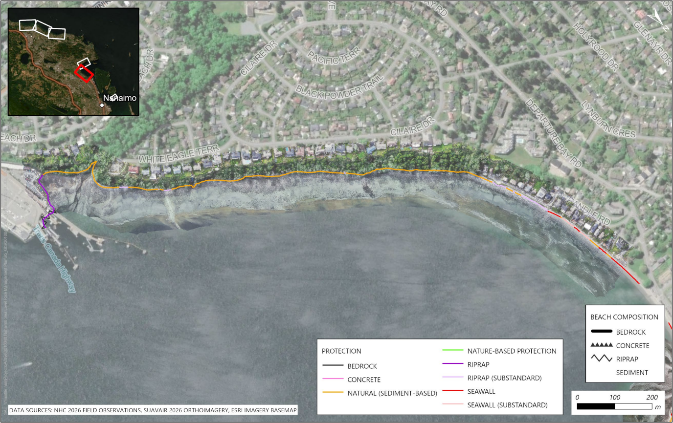
Figure 3.14 Shoreline protection and beach composition mapped along the Cilaire focus area.
