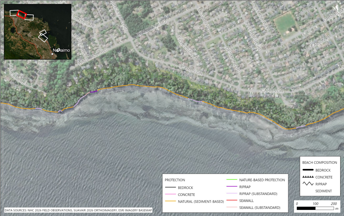
Figure 3.6 Shoreline protection and beach composition mapped along the center of the North Shore focus area.
