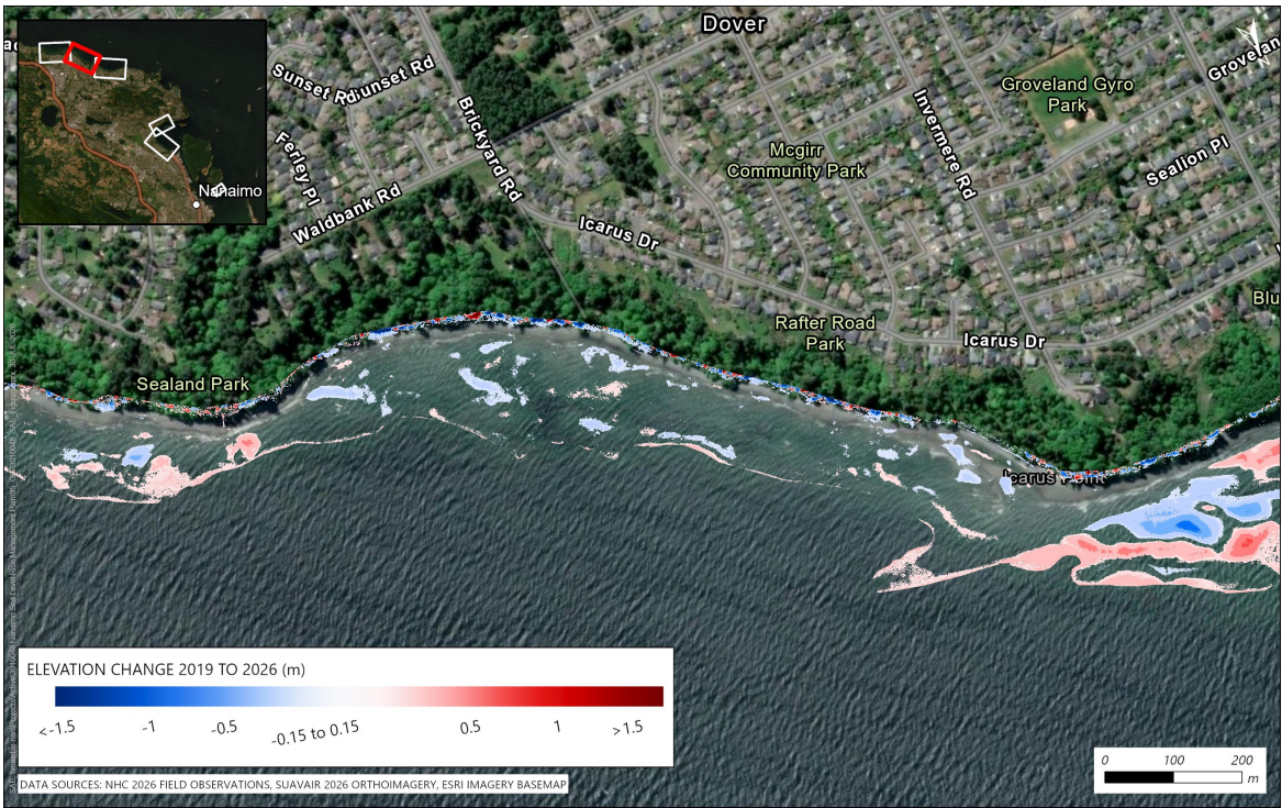
Figure 3.25 Elevation change at the center of the North Shore focus area between 2019 (GeoBC Lidar) and 2026 (SuavAir Drone Survey Lidar).
