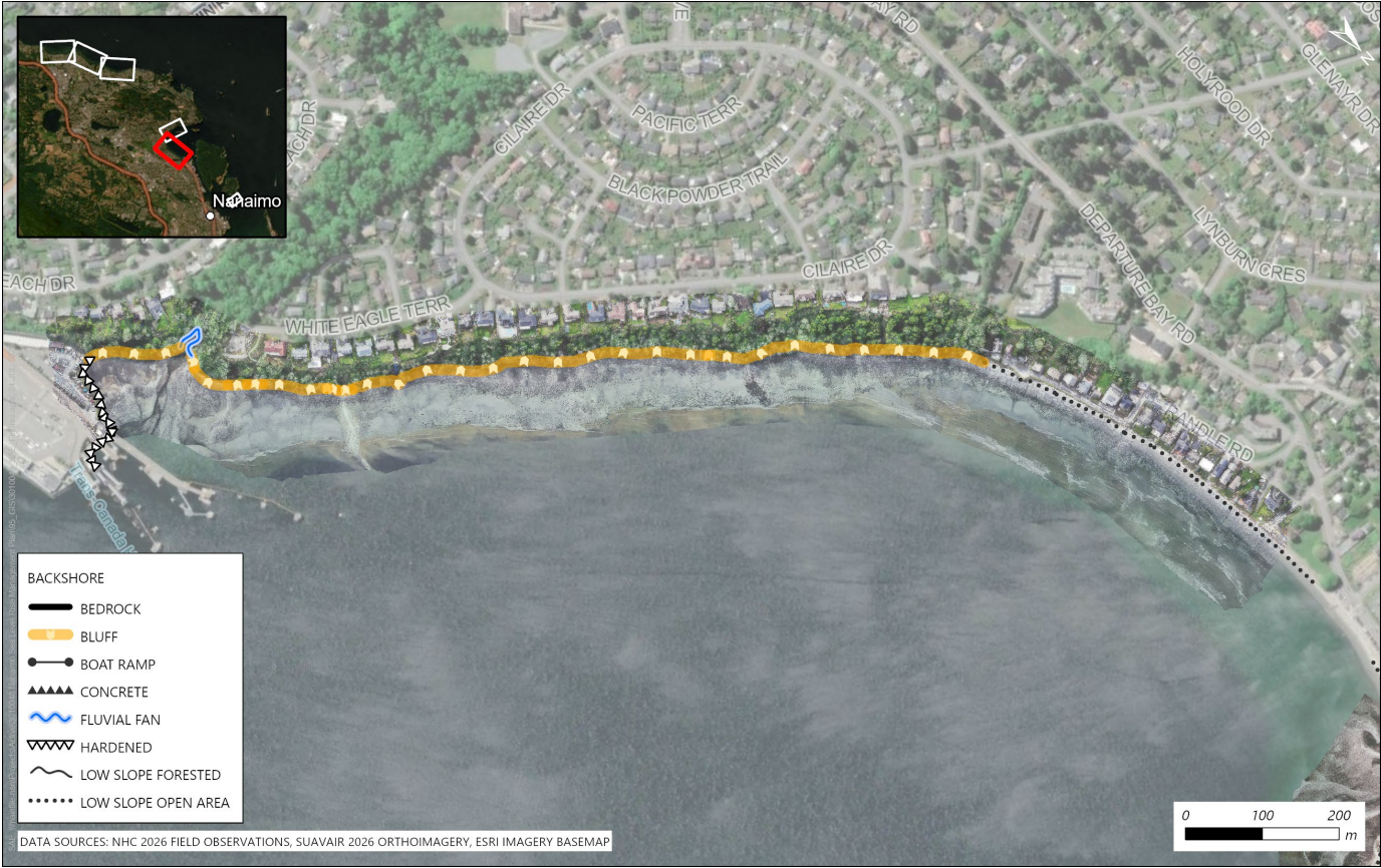
Figure 3.15 Backshore morphology mapped along the Cilaire focus area.
