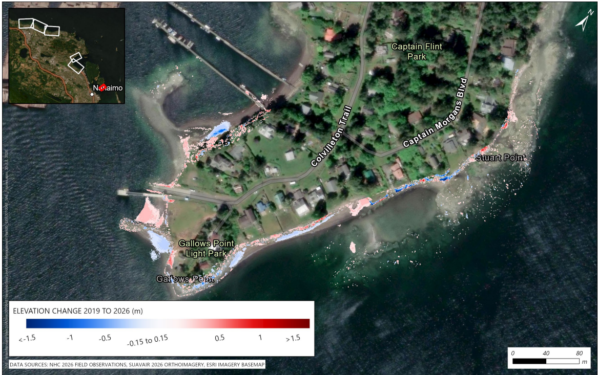
Figure 3.29 Elevation change at the Protection Island focus area between 2019 (GeoBC Lidar) and 2026 (SuavAir Drone Survey Lidar).
