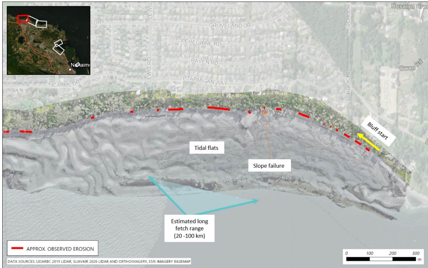
Figure 3.1 Map of observed features and areas of active erosion along the west side of the North Shore focus area. Slope failure location is approximate.
