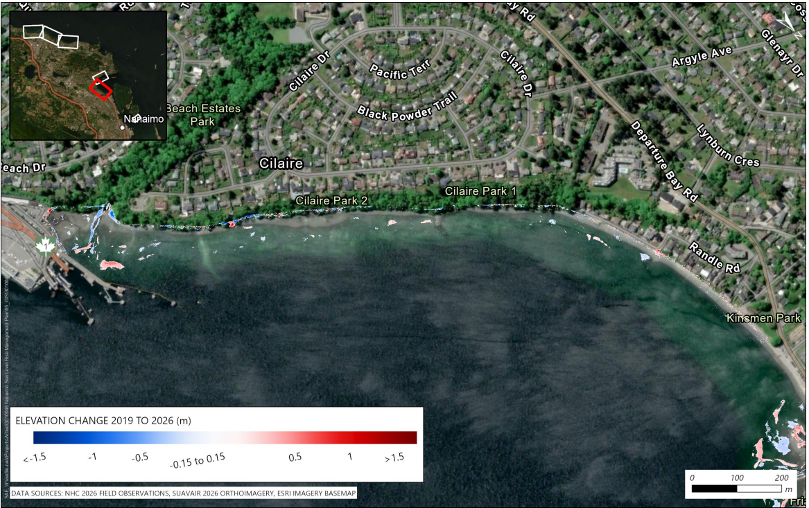
Figure 3.28 Elevation change at the Cilaire focus area between 2019 (GeoBC Lidar) and 2026 (SuavAir Drone Survey Lidar).
