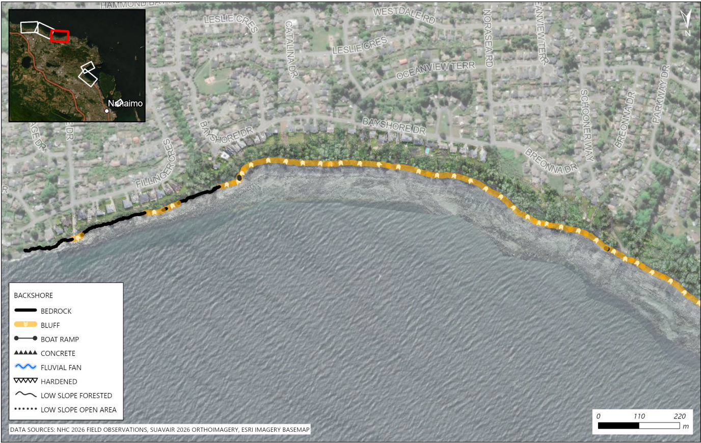
Figure 3.9 Backshore morphology mapped along the east side of the North Shore focus area.
