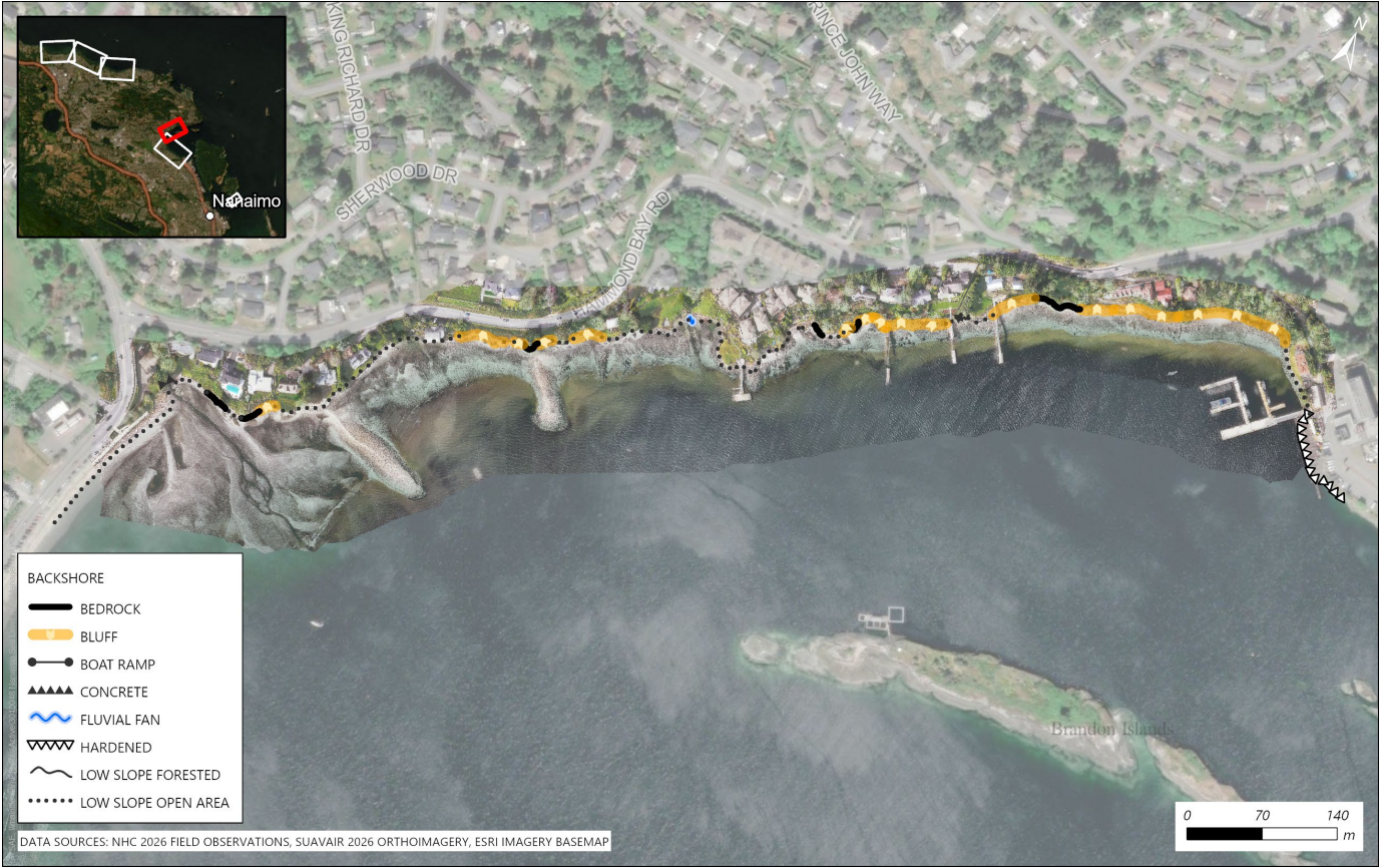
Figure 3.12 Backshore morphology mapped along the Departure Bay focus area.
