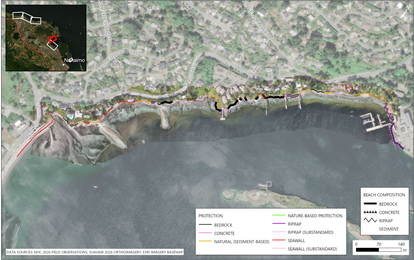
Figure 3.11 Shoreline protection and beach composition mapped along the Departure Bay focus area.
