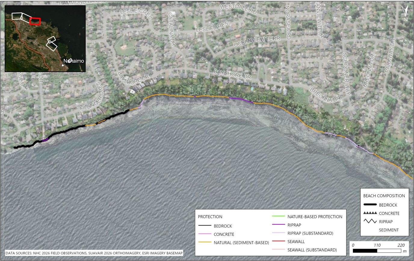
Figure 3.8 Shoreline protection and beach composition mapped along the east side of the North Shore focus area.
