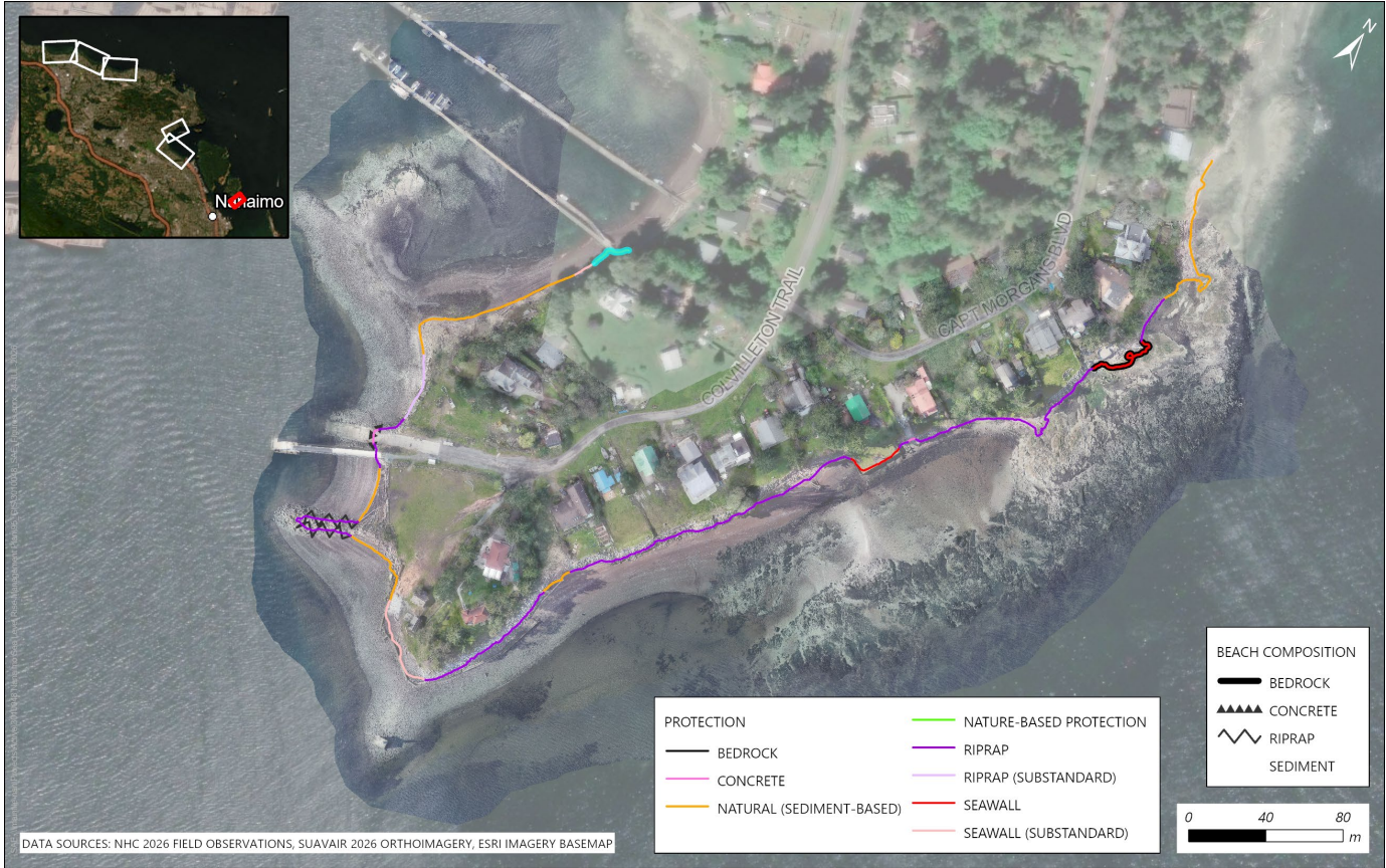
Figure 3.17 Shoreline protection and beach composition mapped along the Protection Island focus area.
