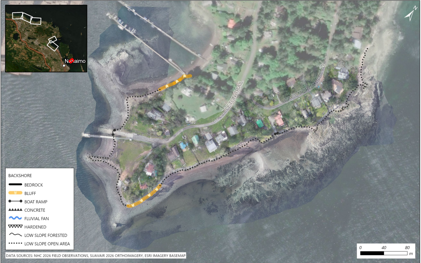
Figure 3.18 Backshore morphology mapped along the Protection Island focus area.
