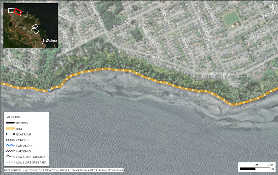
Figure 3.7 Backshore morphology mapped along the center of the North Shore focus area.
