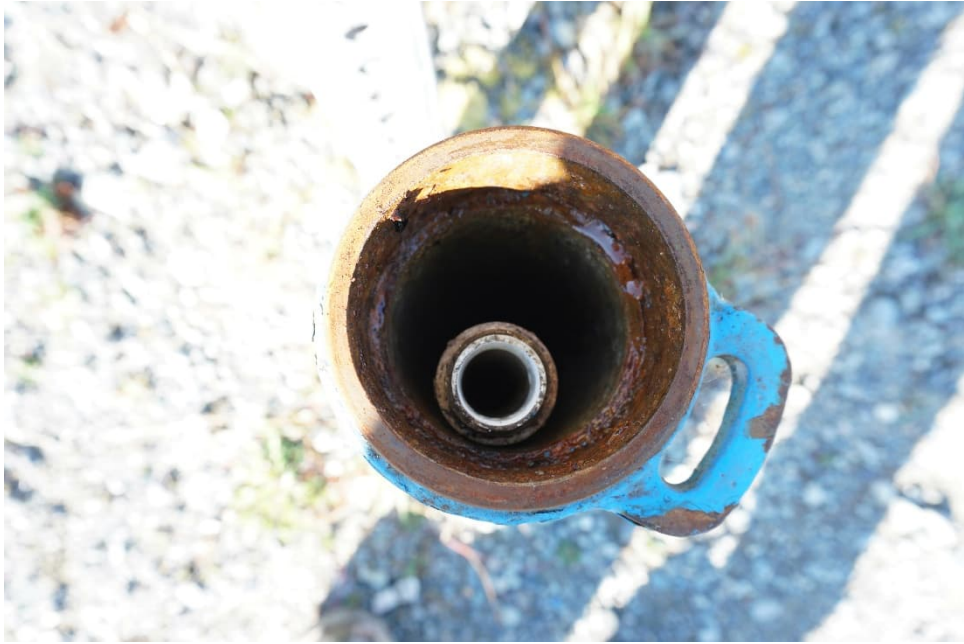
JCR 25: Typical Standpipe Piezometer within Casing
