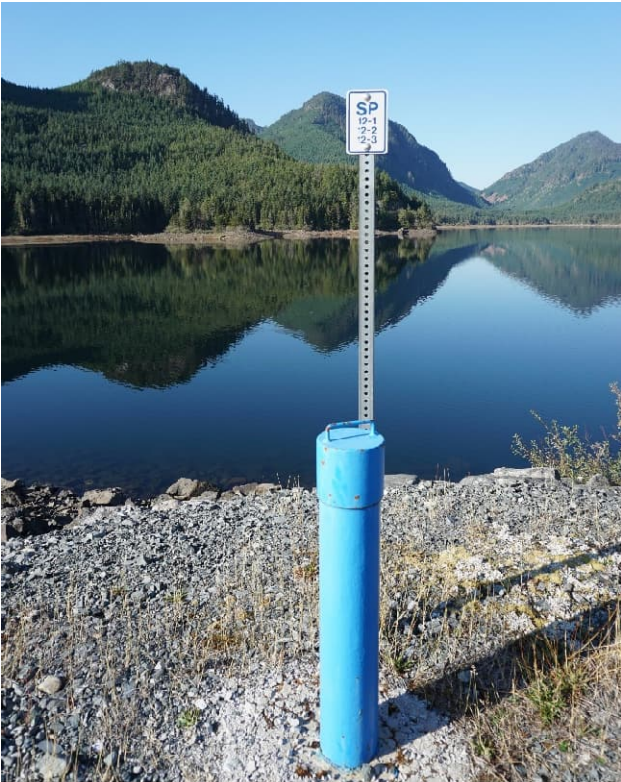
JCR 24: Typical Standpipe Piezometer Casing
