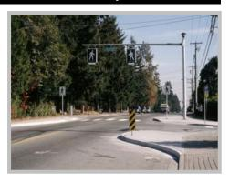
**Benefits:** Curb extensions improve pedestrian safety by reducing the crossing distance, and by improving visibility for both approaching motorists and waiting pedestrians. In addition, curb extensions on one or both sides of the roadway may also help to reduce vehicle speeds. For this purpose, curb extensions may be built on either urban or rural roadway cross sections.
