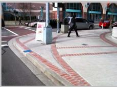
down right-turning vehicle speeds by making the corner 'tighter' with a smaller radius. A corner radius reduction may also improve pedestrian safety to a certain degree by shortening the crossing distance.
