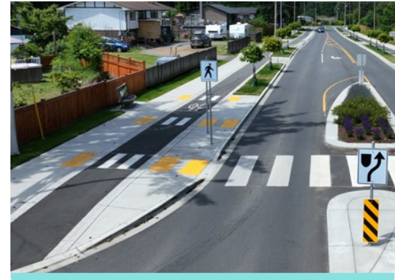
Metral Drive, Nanaimo. In a traditional floating bus stop, the cycle track surface continues in asphalt, with TWSIs, signage, and road markings to indicate pedestrian right-of-way.
