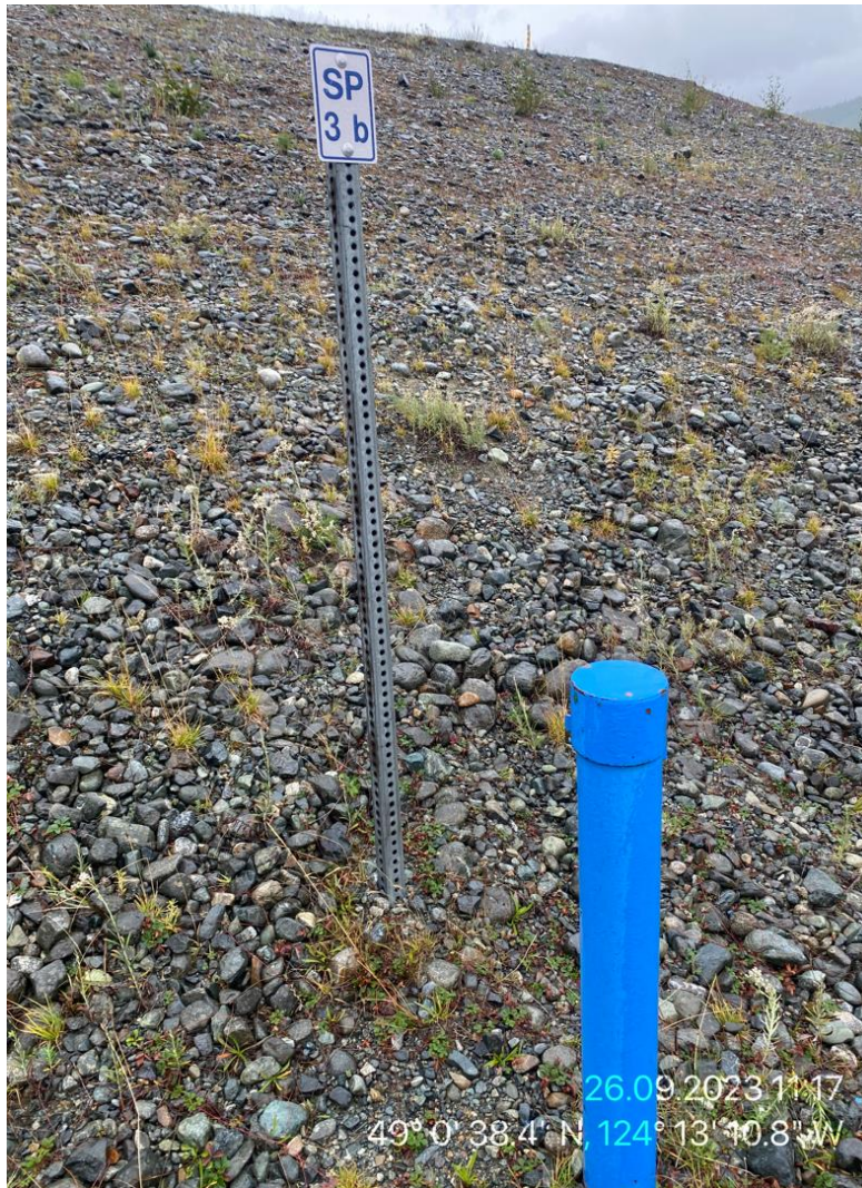
JCR 25: Typical Standpipe Piezometer Casing (SP 3 b)
