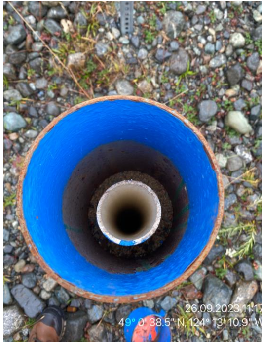
JCR 26: Typical Standpipe Piezometer within Casing (SP 3 b)
