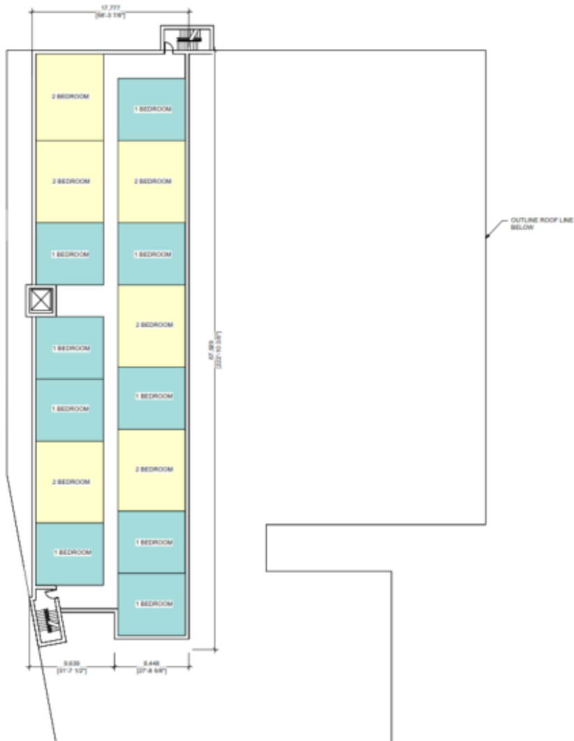
Figure 18 – Optional Housing above Community Centre Third and Fourth Floor Plans at preferred site
