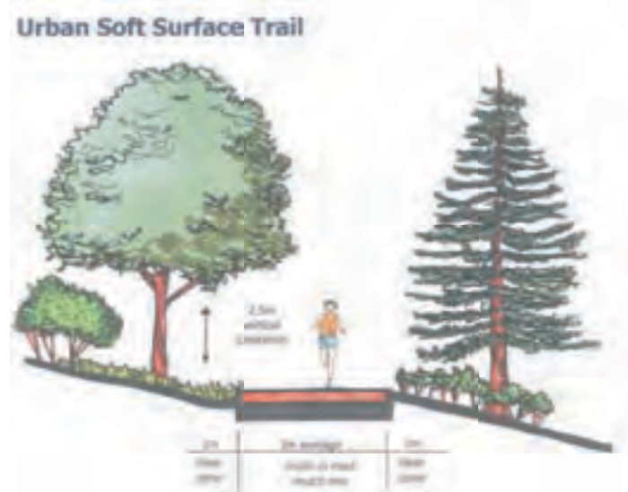
TYPICAL TRAIL SECTION SCALE 1:150
