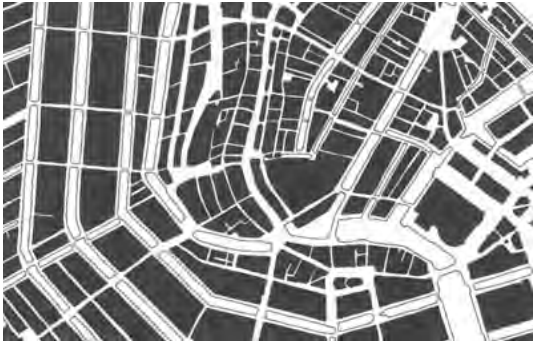
FIGURE GROUND - Urban design tool to study built versus unbuilt urban areas.
