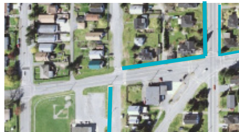
Plan of disconnected pedestrian realm (existing sidewalks shown as blue line)
