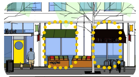
Tall, narrow shopfronts help to break up larger building forms and create a visually interesting rhythm along the street.
