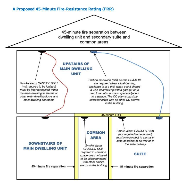
Note: Some smoke alarms may be combination units that include carbon monoxide alarm. Wireless technology is acceptable for interconnecting smoke alarms & interconnecting CO alarms in houses with secondary suites. Each smoke alarm must be installed with a permanent electrical connection. Carbon monoxide alarms do not require a permanent electrical connection.
