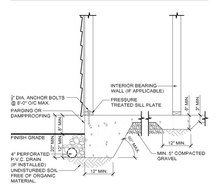
FOR NON-INSULATED, NON-HEATED ACCESSORY BUILDINGS UNDER 55m<sup>2</sup> (592ft<sup>2</sup>) ONLY
