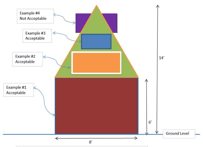
There will be a maximum sign size of 48 square feet at ground level. There is a maximum sign height of 14'. Once the sign reaches this height or exceeds the borders noted on the diagram, a Structural Engineer would be required to design and oversee the installation. This is a general policy. This does not take into account interior designs of support structures for the signage.
