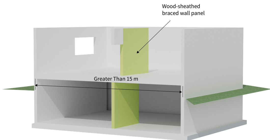
Figure 3.8: Braced Wall Panels in the Basement
