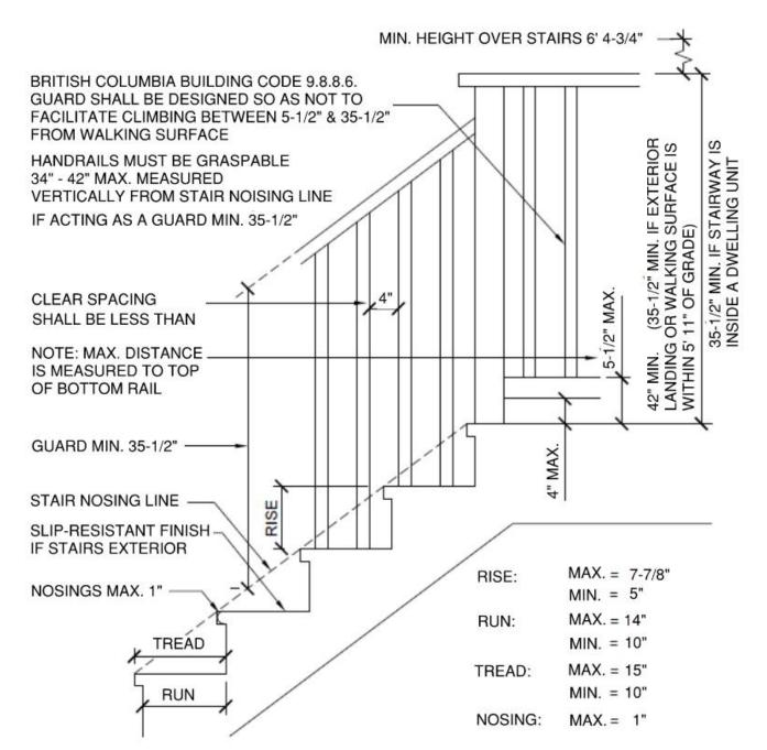
STAIR WIDTH: MIN. 34" CLEAR ONE HANDRAIL REQUIRED ON EXTERIOR STAIRS WITH MORE THAN THREE RISERS AND INTERIOR STAIRS WITH MORE THAN TWO RISERS SERVING NOT MORE THAN ONE DWELLING UNIT
