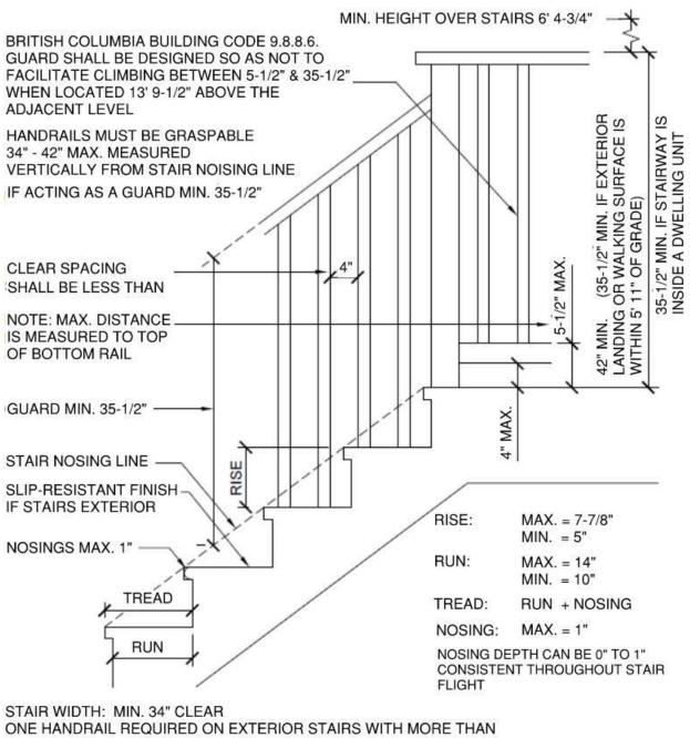
ONE HANDRAIL REQUIRED ON EXTERIOR STAIRS WITH MORE THAN THREE RISERS AND INTERIOR STAIRS WITH MORE THAN TWO RISERS SERVING NOT MORE THAN ONE DWELLING UNIT
