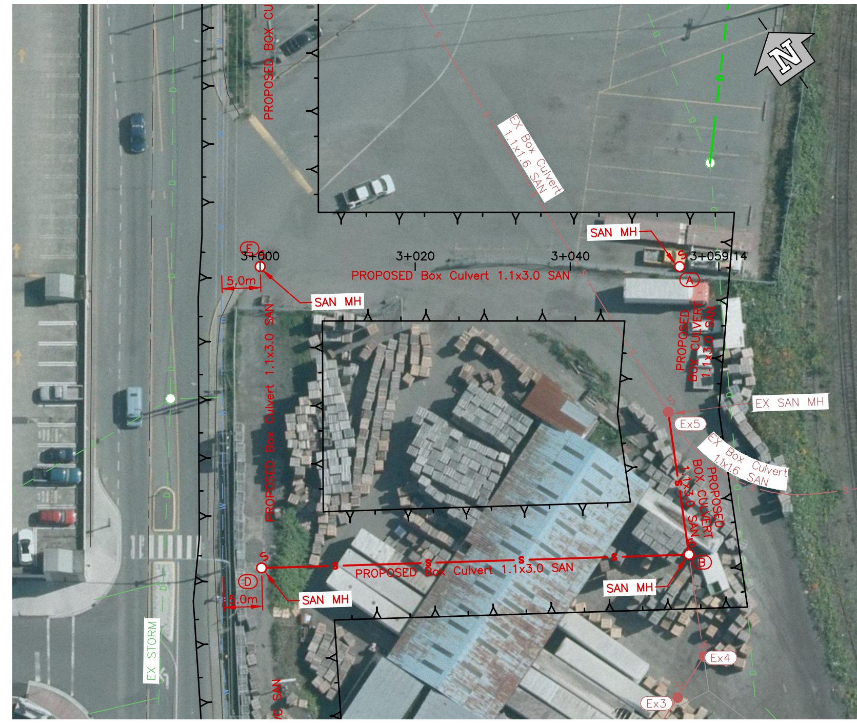
SANITARY REROUTING – OPTION 1 SCALE 1:500
