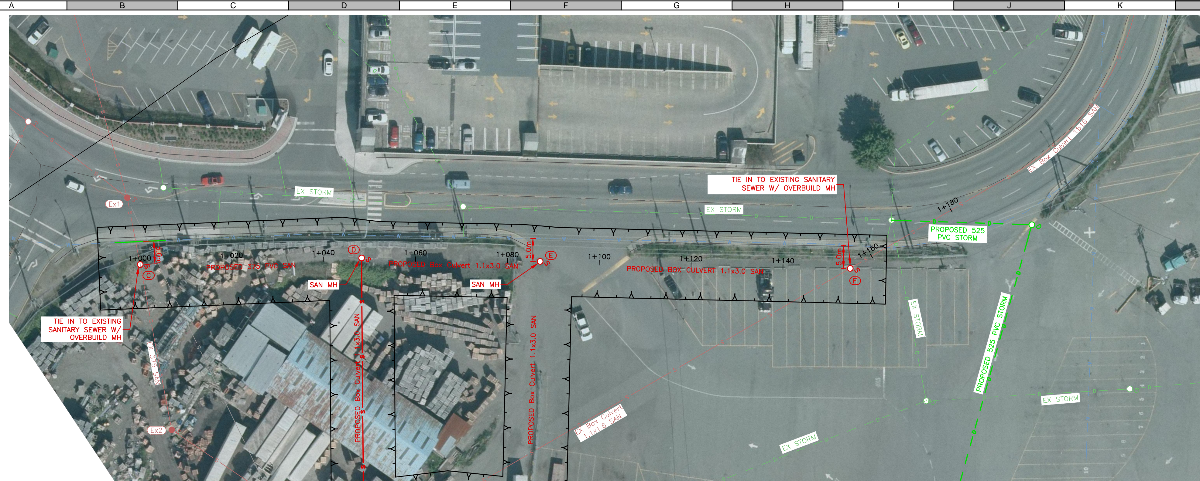
SANITARY REROUTING - OPTION 1 SCALE 1:500
