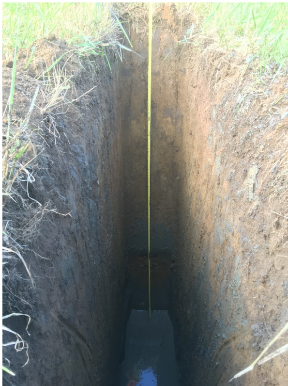
Photo 4. Physical measurements of the soil profile and depth to water.
