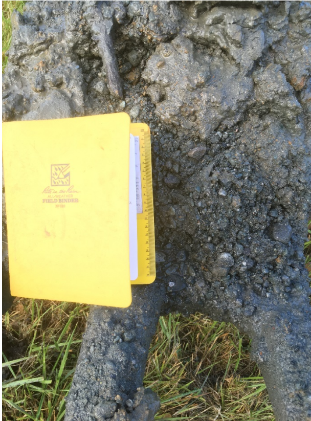
Photo 6. Sand and gravels from the bottom of the Well #1 excavation.
