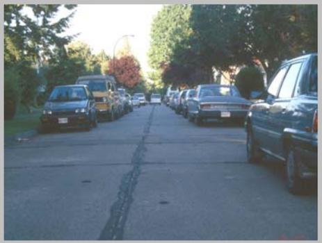
**Benefits:** The primary benefit of allowing on-street parking as a traffic calming measure is the reduction in vehicle speeds due to the narrowed travel space. Also the parked cars act as a buffer between traffic and pedestrians.
