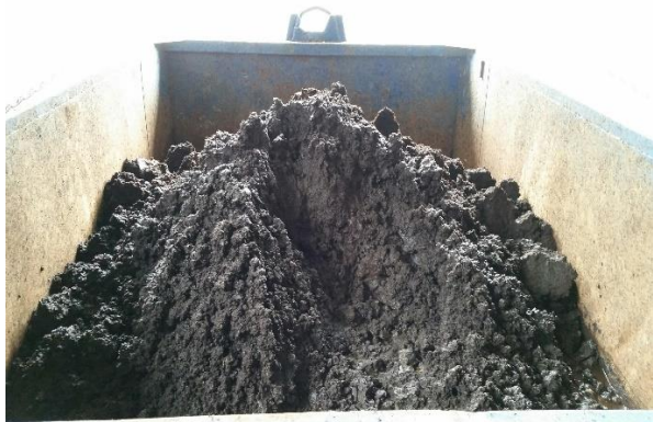
Dewatered sludge (dirt removed from water by centrifuge) ready for disposal
