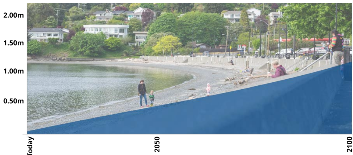
Figure 4: Recommended sea level rise allowances from present day to 2100 (figure adapted from the Province of BC)
