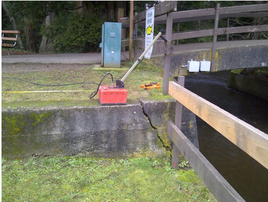
Photograph B-4: Lower Dam—from The Peninsula looking east, adjacent to the spillway (on the right). The red box on top of the retaining wall is the 400 MHz GPR antenna at the south end of line L-9.
