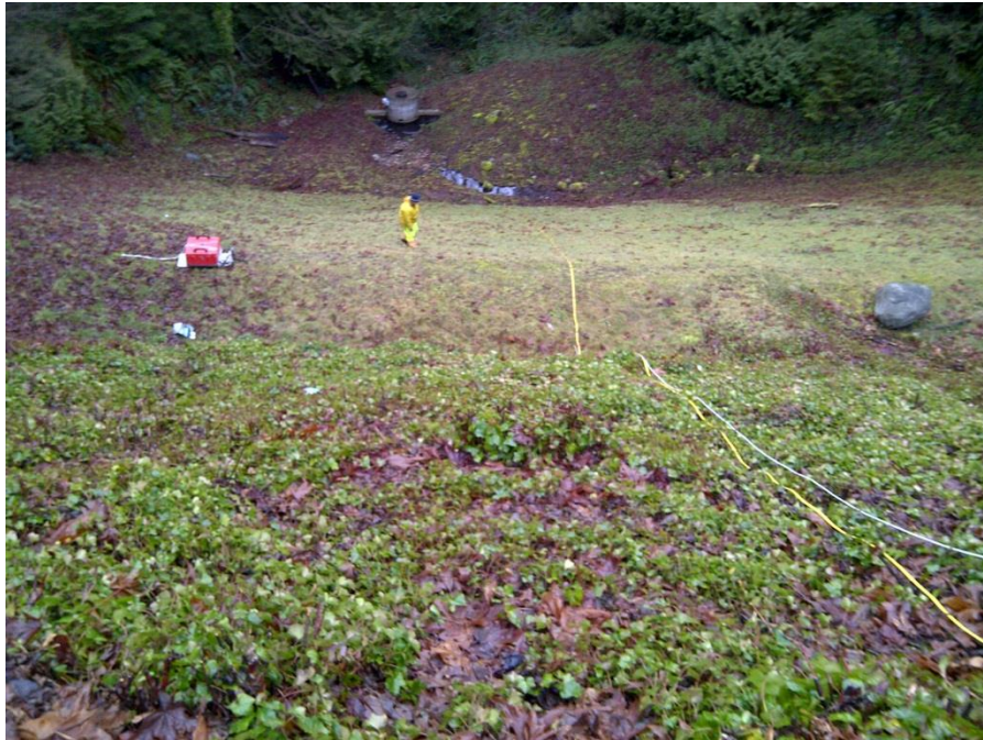
Photograph B-1: Lower Dam—looking down geophysical line L-1 from the dam crest. The red box staged on the berm bench is the 200 MHz GPR antenna.
