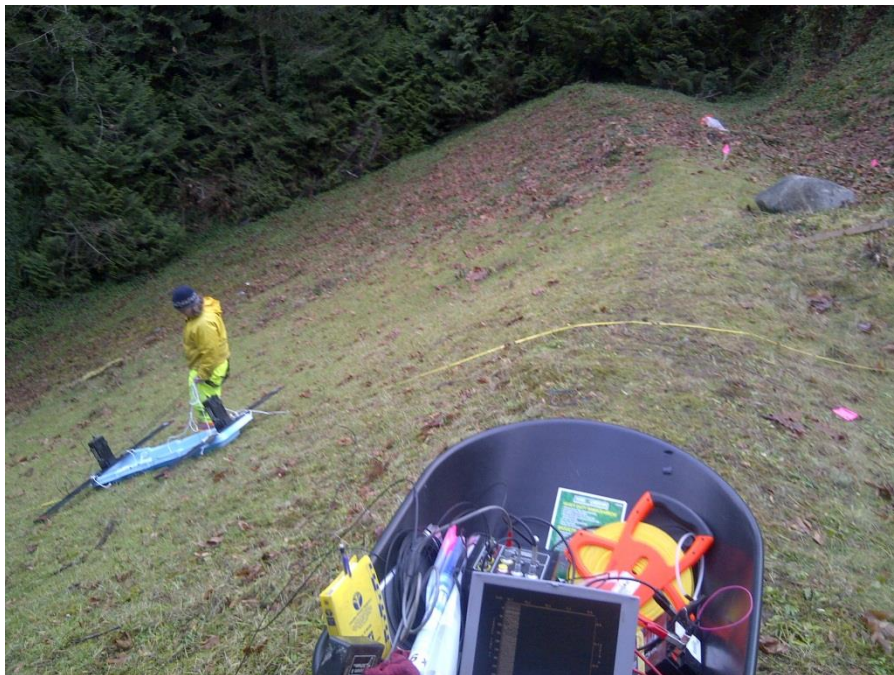
Photograph B-3: Lower Dam—from the toe-berm bench, looking south with the high powered GPR electronics in the wheelbarrow and the 50 MHz antennas profiling on line L-1.
