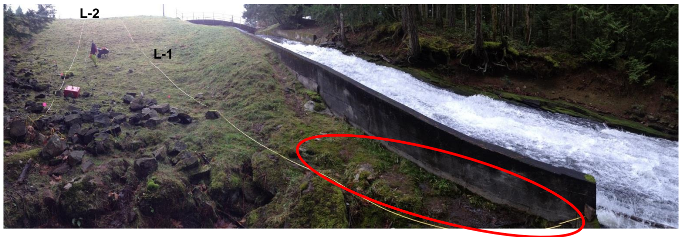
Photograph B-6: Middle Dam—looking up from concrete weir. Lines L-1 and L-2 are marked by the measuring-tapes. Bedrock outcrop occurs within the red circled area and spans the floor of the spillway. The red box on L-2 is the 200 MHz GPR antenna.
