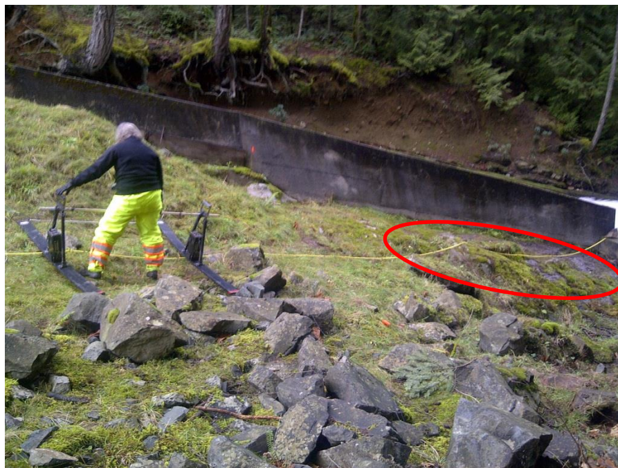
Photograph B-8: Middle Dam—High-powered 50 MHz antennas on line L-1. Bedrock outcrop occurs within the red circled area and spans the floor of the spillway.
