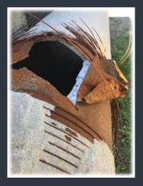
A large watermain break to an in-town water supply main in April 2020 caused significant damage, loss of water to many businesses, residents and jeopardized the City's water supply and fire fighting capabilities.
